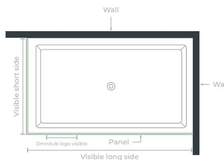
This panel is manufactured as one whole piece and is to be used on an Omnitub® bath tub where the visible long side of the bath tub connects to the visible short side on the left hand-side.
