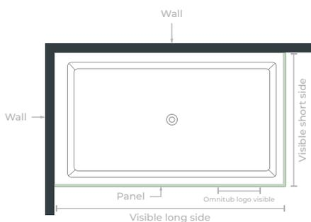
This panel is manufactured as one whole piece and is to be used on an Omnitub® bath tub where the visible long side of the bath tub connects to the visible short side on the right hand-side.
